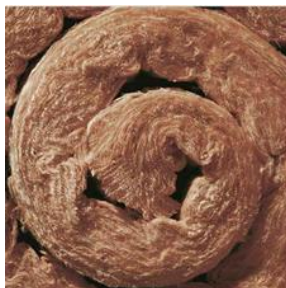
Porous, mineral wool absorber
