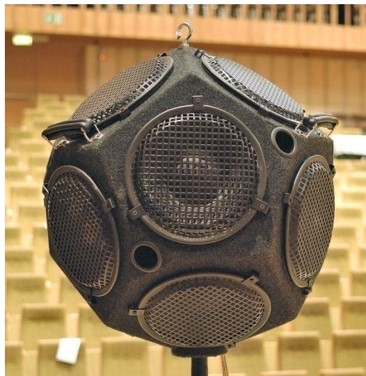
Fig 7.2. View of the typical omnidirectional source made of 12 loudspeakers, mounted on the surface of dodecahedron.
